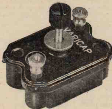
R.I. "Varicap" semi-variable condensers with a maximum capacity of 0.001 mfd.
