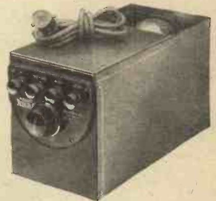
Clarke's "Atlas" A.C. battery eliminator. Model A.C. 16.
