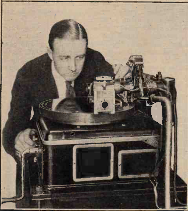
Fig. 4.—"Wax" disc on recording machine, showing recording expert cutting an original record. Note the mirror reflection in the polished "wax," also the air-suction pipe to exhaust the shavings.
